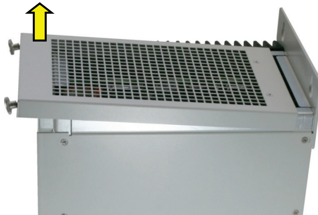
Figure 35: Removing the cover (detail of the KBox C-102-2)
