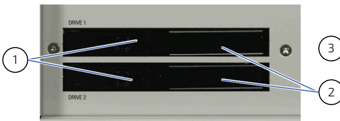
Figure 20: Drive 1 and Drive 2 for removable 2.5" SATA HDD/SSD (option); closed drive bays
