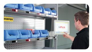
With the central Panel PC as the main user interface, the i-Pick can achieve a pick performance of 600 lines/hour and a 300% increase in efficiency, combined with a 10-fold rise in the order-picking quality compared with conventional order-picking methods.
