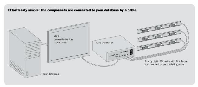
The i-Pick system consists of 4 main components: Pick by Light (PBL) rails with pick faces. The Line Controllers that can handle up to 200 pick faces and the panel PC that is the central user interface that is usually in direct interaction with a central SQL database and serves XML data files via USB, wireless or wired LAN.
